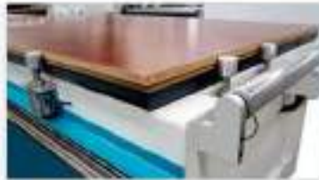
Pop-up pins for accurate positioning of workpiece
