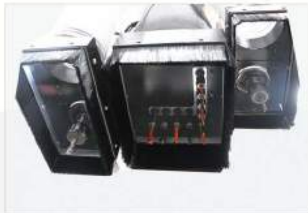
Two spindles, one for resting, one for grooving, or have it your way—the two manual tool changing spindles work together and eliminates half the tool-changing time. 5+4 Vertical Drill Bank is standard feature.
