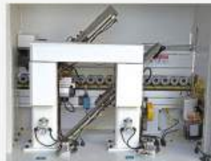
Two motors traveling on linear guides for end-trimming
